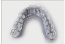
**3. VACUUM FORM**Using an intermediary/separator layer, vacuum form over the 3D print using a pressure former.
