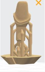
Printing on supports is also possible, and is recommended in cases where dies have small pin diameters (less than 3 mm).
