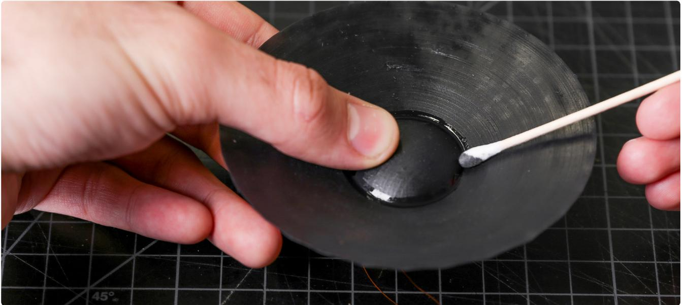
The cone is designed to be extremely thin, making it as light as possible while staying rigid. The cone's thickness is tapered down to 0.3 mm at the edge.
