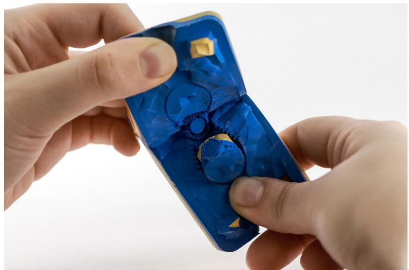
*Interior of natural rubber mold, made with master printed on the Form 2 with High Temp Resin.*
