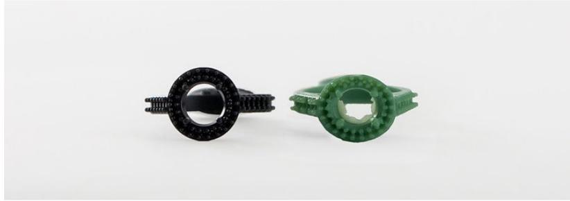
The original shape of the halo ring printed in Black Resin (left) distorted when exposed to high temperature vulcanization, yielding a misshapen mold and poor quality molded waxes (right). This was not a problem when using High Temp Resin, which has a higher Heat Deflection Temperature (HDT).
