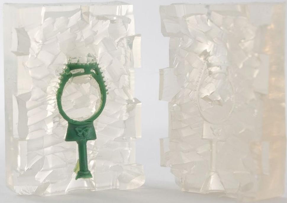
*Master pattern, printed on the Form 2 in Black Resin, and silicone mold with molded wax.*
